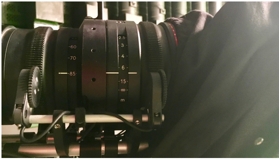
Figure 6: Lens encoder for zoom and focus.
