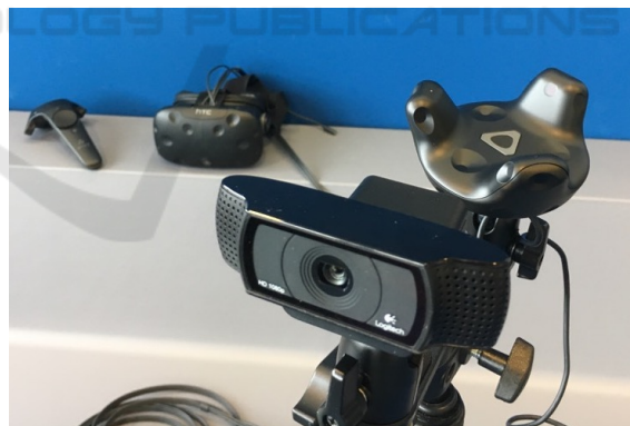
Figure 5: Webcam with lower delay with Vive tracker.
