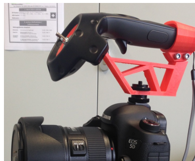
Figure 4: DSLR camera with Vive controller and custom-printed adapter.
