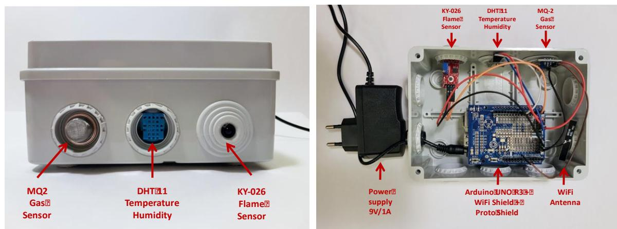
Figure 2: Smart Device Prototype Implementation.
