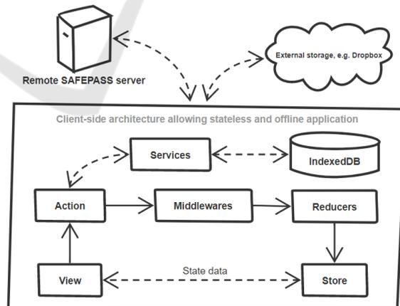
Figure 2: Low level client architecture with Flux.
