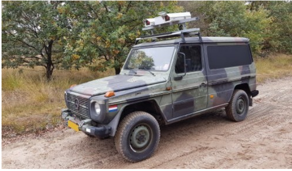
Figure 8: Prototype vehicle used for our experiments, featuring a stereo camera with 1920 \times 1440 pixel resolution and a GPS/IMU positioning system for georeferencing the images.
