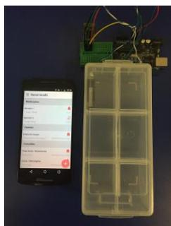
Figure 2. Prototype of the medication smart box to be connected with Renal health application.
