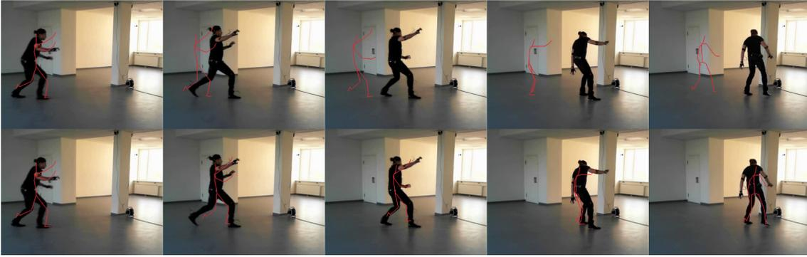
Figure 7: Comparison of XSens MVN tracking (top) and our optical-inertial evaluation (bottom). In the second frame, the sliding starts and the mocap system fails to evaluate the position correctly. Images were captured using a Microsoft LifeCam HD 3000 RGB webcam.
