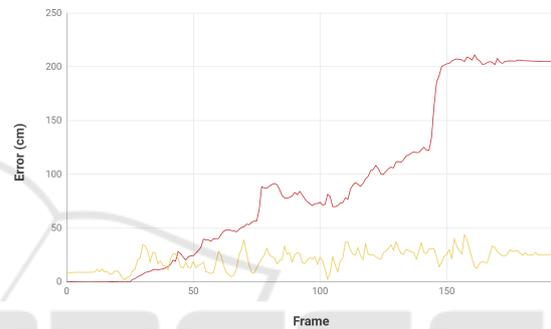
Figure 8: Comparison of error difference in Euclidean distance between the methods and ground truth obtained using HTC Vive: (Red) original position from inertial suit software and (yellow) our optical-inertial method. Graph is evaluated on a dataset, where the movement was the most problematic for the original method (e.g. jumping, sliding).
