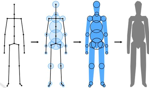
Figure 4: A base mesh is created using the skeleton acquired from the mocap suit. The skeleton is enhanced with measured radii of the actor's body. Note that the base mesh construction process is depicted in 2D only.
