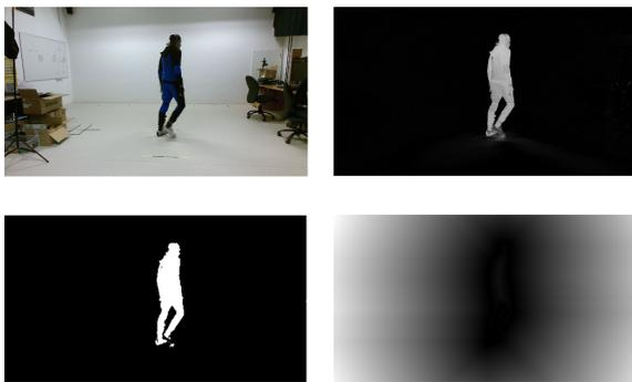
Figure 6: Tracking of the actor position using Chamfer matching. (Top) an input image and the subtracted background image in grayscale. (Bottom) applied adaptive thresholding and calculated distance transform of the silhouette.
