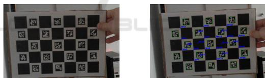
Figure 1: The ChArUco calibration board. The ChArUco is a combination of the classical calibration checkerboard and the ChArUco alphabet signs.
