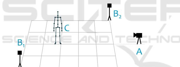
Figure 10: The evaluation setup. The subject wearing a mocap suit (C) is captured by a camera (A) and tracked by HTC Vive lighthouses (B). The position estimated by the lighthouses is used as a ground truth when the original mocap suit tracking is compared to the proposed method.
