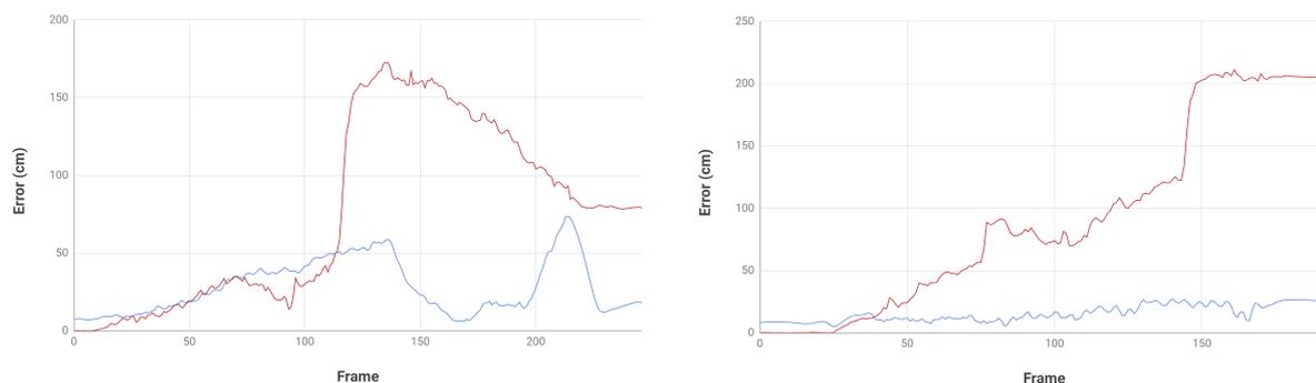
Figure 9: Comparison of error difference with filtered data: (Red) position calculated by original inertial suit software and (blue) post-processed versions of estimated positions using our approach. Another example from the datasets is plotted on the right. In both cases, the smoothed versions of evaluated positions approximate the movement and the real position of the subject much better.
