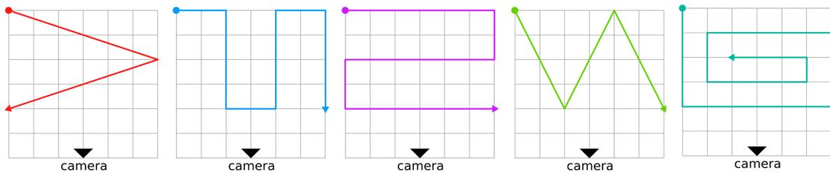
Figure 11: Evaluation of our method on different trajectories within a grid. The grid has a size of  $6 \times 6$  meters. The patterns were chosen to fully cover the tracking area in different directions. Moreover, different types of movement were used during the evaluation, such as walking, jumping, sliding etc.
