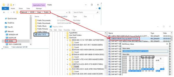
Figure 3: Artifacts of program run from a shared network in UserAssist key.
