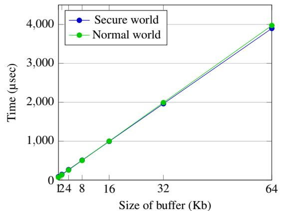
Figure 5: Mean execution times for SHA-256 hashing a variable sized buffer in the Secure world, compared to hashing in the Normal world.
