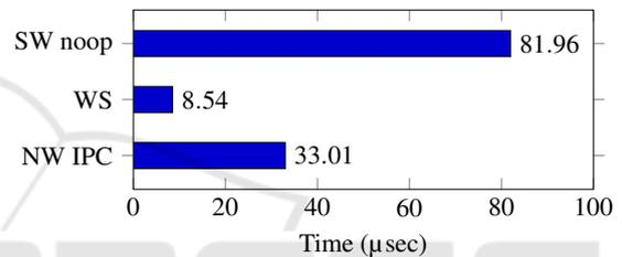
Figure 3: Mean end-to-end execution times for a noop Secure world invocation executed 1000 times, compared to traditional IPC between Normal world processes through named pipes.
