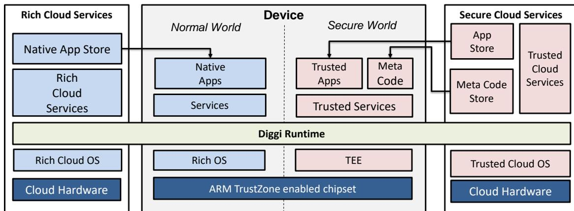
Figure 2: Outline of application provisioning for IoT devices in Diggi. The Normal world part of the application is distributed from a cloud-hosted appstore to the Normal world OS. When the application requests trusted execution or access meta-code protected data, the Secure world will request the secure part of the application through the secure appstore and do validation of the code before installing it and allowing requests between worlds.
