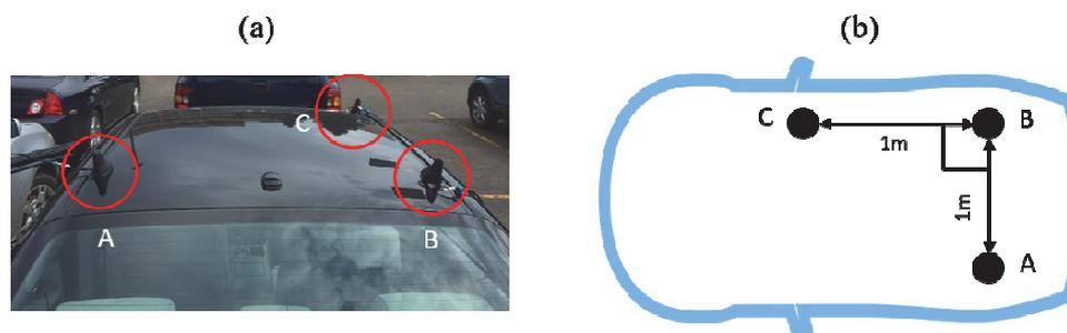
Figure 3: The top view of the vehicle used for the field tests with (a) pictorial view and (b) schematic view, showing three installed antennas and their relative locations.
