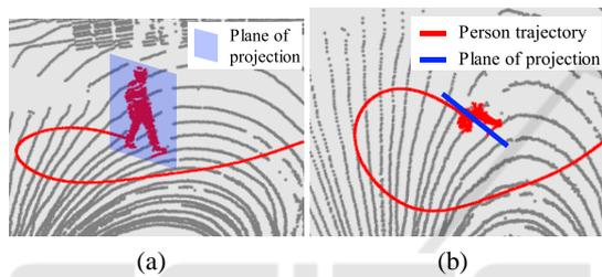
Figure 3: The projection plane for LGEI generation from a) side-view, b) top view.
