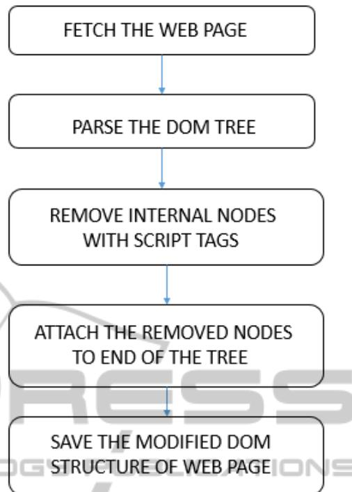
Figure 1: Placing scripts at the bottom of the page.
