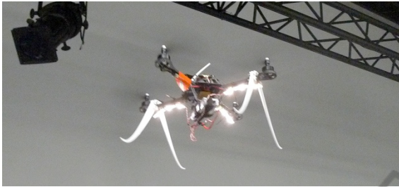
Figure 2: A single Spaxel represented by a quadcopter, an unmanned aerial vehicle with preliminary LED lighting.
