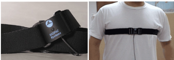
Figure 2: Respiratory effort transducer SS5LB and its location.
