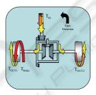
Figure 2: BTV general scheme.  $T_{IN}$ : input torque;  $T_{OUTI}$  and  $T_{OUT2}$ : resultant torque to each output shafts;  $T_{Brake}$ : braking torque.
