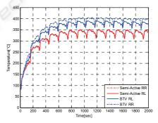
Figure 15: Brake pad temperature estimation.
