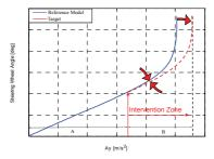
Figure 1: Reference understeer and target diagram.
