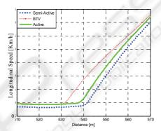
Figure 11: U-turn. Longitudinal speed vs. distance.
