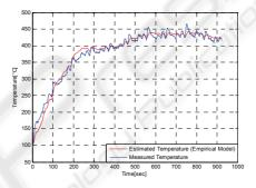
Figure 14: Comparison between measured and estimated braking pad temperatures.
