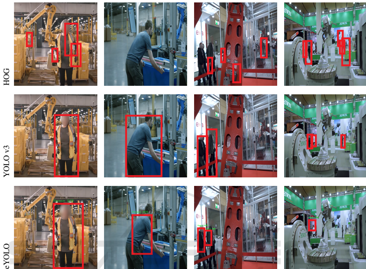
Figure 17: Person detection in typical working scenarios with HOG (top row), YOLO v3 (middle), and eYOLO (bottom).
