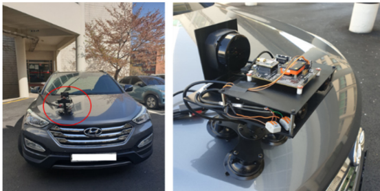
Figure 8: Mobile Mapping System to acquire data of parking spaces and ramp.
