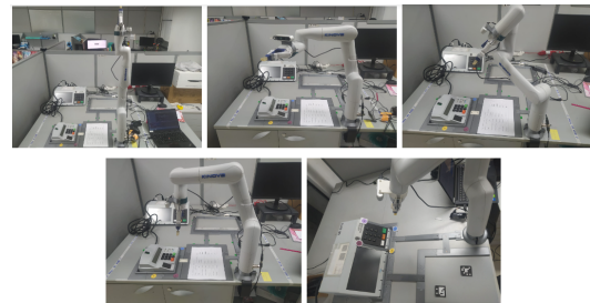
Figure 6: From right to left and from top to bottom, the positions: "0", "Home", movement attempt to "see" from the polling station's terminal, "see" from the polling station's terminal, see from the voter's terminal.
