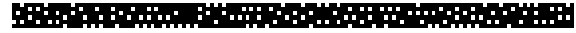
Figure 3: Binary pattern with uniqueness within a window size of 6 \times 6 which is used in the structured light modules. The pattern is repeated horizontally and vertically to fill the entire projector image.
