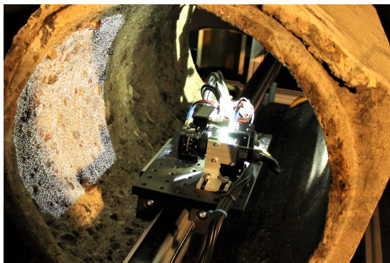
Figure 9: Experimental setup for evaluating the generated 3D point cloud of a real sewer section. Please note that the rig shown was only used to evaluate different camera-projector setups during our research. The final robot is depicted in Figure 2.
