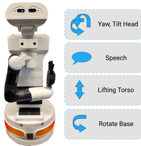
Figure 1: The TIAGo robot platform with the key operations used in our method.
