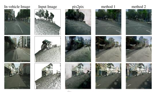
Figure 7: Real image experiments. The rightmost three columns show pedestrian views obtained from in-vehicle images in the leftmost column by using the proposed method and the existing method.
