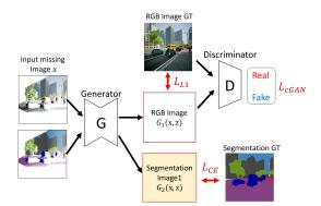
Figure 2: Network structure of method 1. Generator receives missing RGB images and missing label images, and outputs generated RGB images that complement missing RGB images and generated label images that complement missing label images.
