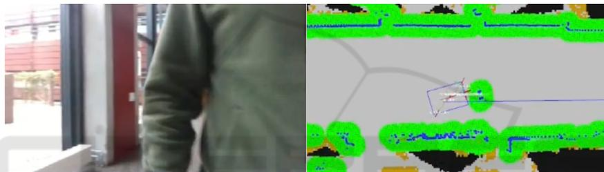
(c) Robot starts to plan local trajectory to avoid collision with the person, but it is too late and the situation end in an emergency stop.
