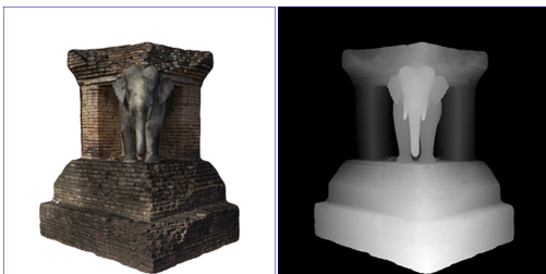
Figure 1: Example of a texture image (left) and its associated depth map (right).
