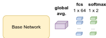
Figure 5: Multi-Task Learning Handcrafted 2 architecture. In purple is the global average pooling layer, in blue the fully-connected layer, and in green the softmax activation.
