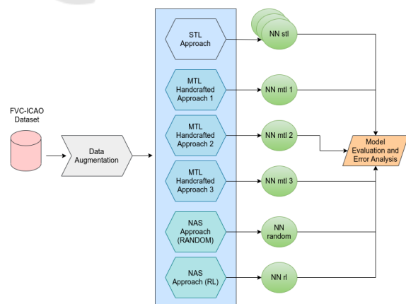
Figure 2: Scheme of the method, specifying the dataset and each approach proposed, which are evaluated with common metrics (accuracy and EER).
