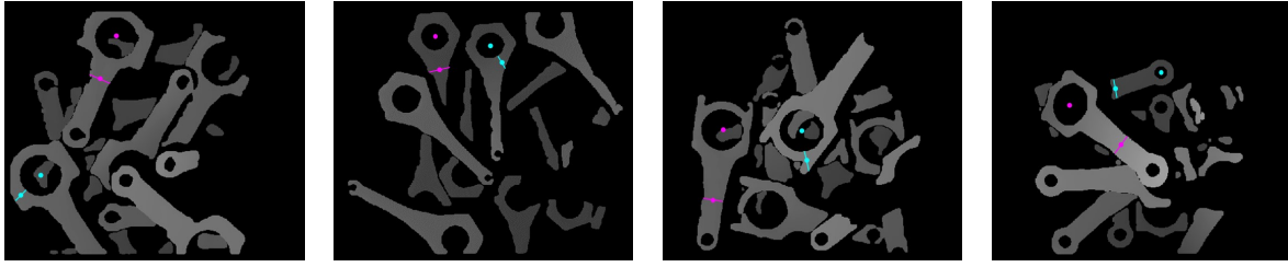
Figure 7: Estimation results of robot motion parameters by the comparison method and the proposed method. The red point shows the result to estimate using the proposed method and the blue point show the result using the comparison method. If robot grasp blue point on the part, assembly will fail because of collision between robot hand and shaft. If the center of gravity of a small hole is estimated as the point of action, it is not possible to insert the part into the shaft. However, the proposed method estimates the optimal robot motion parameters (red point) for assembly.
