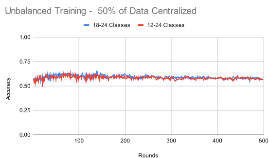
Figure 6: Unbalanced federated training results starting from a centralized model pre-trained with 50% of training data. (blue): The classes vary between 18 and 24. (red): The classes vary between 12 and 24
