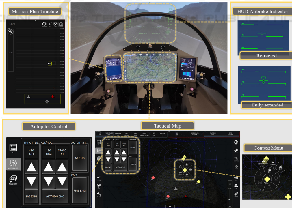
Figure 3: Simulator (top center) with relevant interaction elements: Mission timeline (top left), HUD air brake indicator (top right), autopilot control (bottom left), tactical map (bottom center) and context menu (bottom right)
