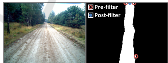
Figure 4: Example of end point filtering which shows both centering end points at road endings and filtering out nearby end points.
