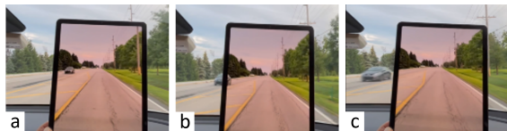
Figure 7: Transparent display frames with passing car moving from being seen on transparent display (a) to being seen directly (c).
