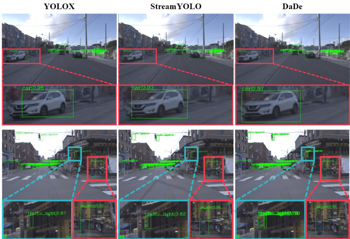
Figure 5: Qualitative analysis of results. Detection is conducted in a streaming environment with a high delay. DaDe can successfully predict the future environment by forming object-moving trends. It achieves better results not only for moving objects (top row) but also for detecting objects during ego-vehicle turns (bottom row).
