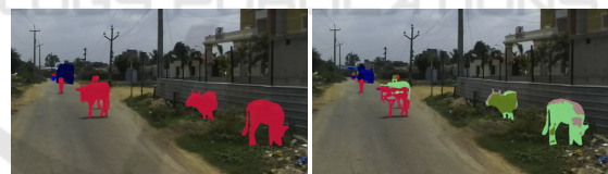
Figure 1: Example image of the India Driving dataset. Left: Ground truth pixels of classes humans/animals colored in red and vehicles in blue. Right: Semantic segmentation for the mentioned classes.
