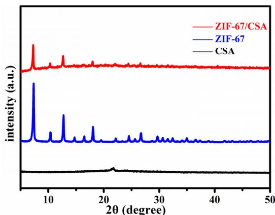
Figure 2: The XRD of CSA, ZIF-67 and ZIF-67@CSA.
