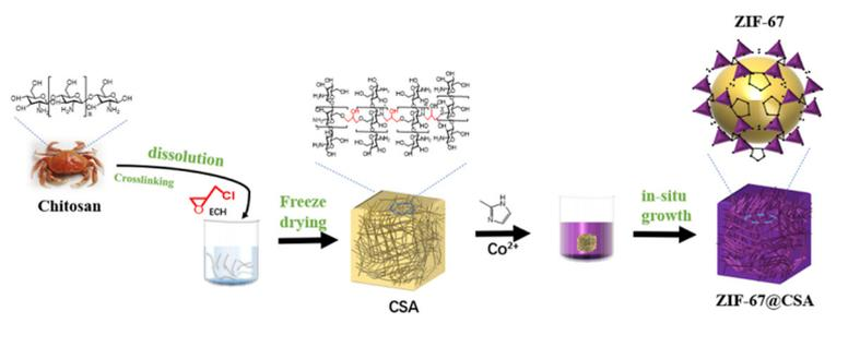
Figure 1: Schematic fabrication process of ZIF-67@CSA.
