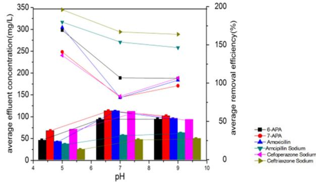
Figure 4: Different contaminants' average removal efficiency and average effluent concentration under different pH.
