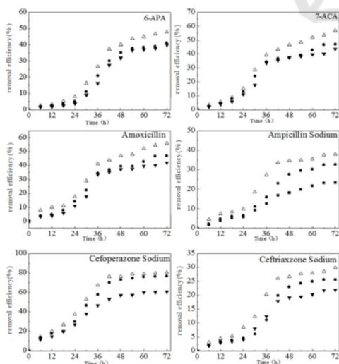
Figure 2. Different target contaminants' removal efficiency in different carbon system.
