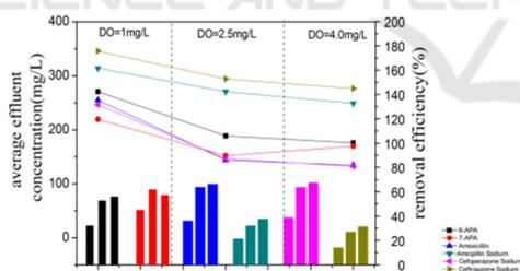
Figure 7: Different contaminants' average removal efficiency and average effluent concentration under different DO (points represented concentration, columns represented removal efficiency).
