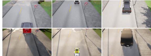
Figure 2: Overview of the different datasets. Upper row 4m camera height. Lower row 3m camera height. The columns show an 45°, 50° and 60° camera pitch from left to right.
