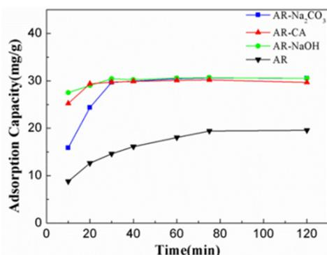
Figure 4: The effect of adsorption time on the adsorption capacity of residue-based bio-adsorbent in Astragalus.
