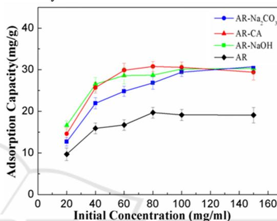
Figure 3: The effect of initial solution concentration on the adsorption capacity of residue-based bio-adsorbent in Astragalus.
