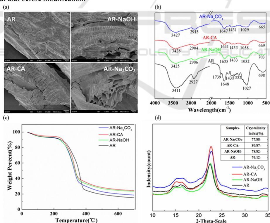
Figure 1: Characterization of AR, AR-NaOH, AR-Na<sub>2</sub>CO<sub>3</sub> and AR-CA. (a) Electron micrographs of AR, AR-NaOH, AR-Na<sub>2</sub>CO<sub>3</sub> and AR-CA. (b) Infrared spectra of AR, AR-NaOH, AR-Na<sub>2</sub>CO<sub>3</sub> and AR-CA. (c) TG results of AR, AR-NaOH, AR-Na<sub>2</sub>CO<sub>3</sub> and AR-CA. (d) XRD results of AR, AR-NaOH, AR-Na<sub>2</sub>CO<sub>3</sub> and AR-CA.
