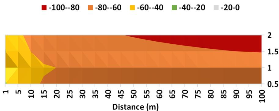
Figure 3: Coverage of AP deployed at a height of 0.5m for each of the emitter heights.
