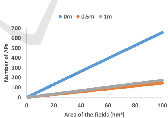
Figure 9: Number of APs per area of the field for the emitter at 2 m.
