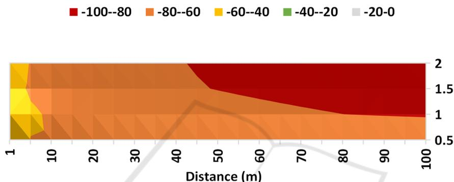
Figure 4: Coverage of AP deployed at a height of 1m for each of the emitter heights.
