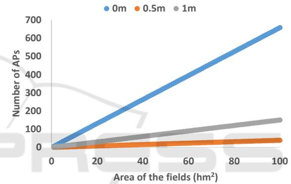
Figure 8: Number of APs per area of the field for the emitter at 1.5 m.
