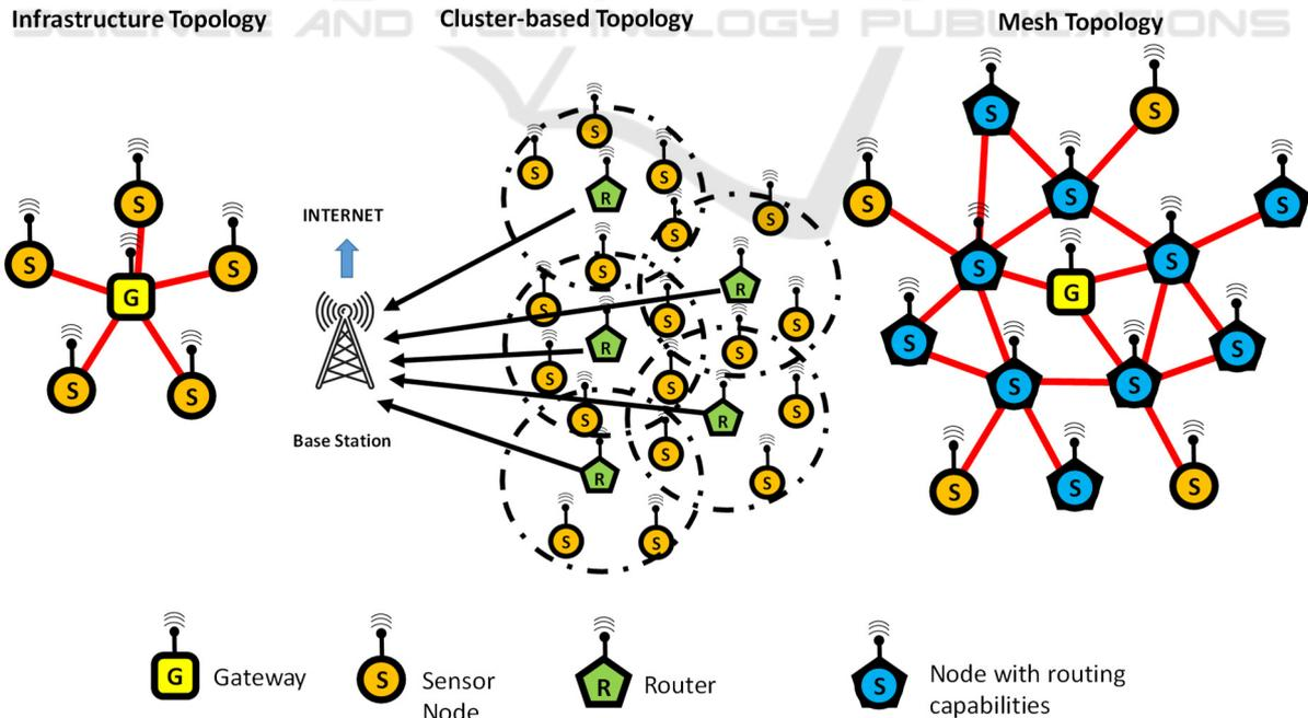
Figure 1: Topologies used in WSNs.
