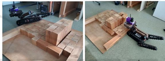
(a) Real robot overcomes 20 cm barrier (begin). (b) Real robot overcomes 20 cm barrier (end).
