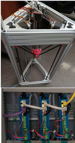
Figure 6: Picture of the Kossel machine used for experimental testing (top) with Nanotec C5E servo-stepper drives (bottom).
