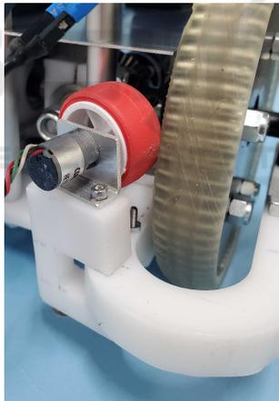
Figure 9: The rotary encoder attached to wheel via roller.
