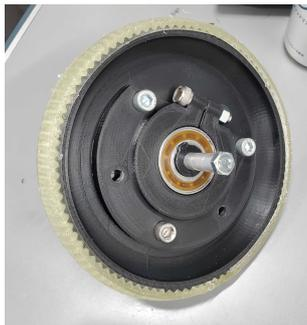
Figure 8: The wheel assembly.
