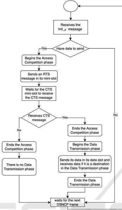
Figure 5: DSNCP flow graph for the edge nodes.
