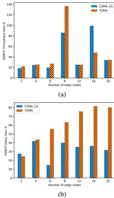
Figure 12: The DSNCP's Delay and Throughput gains compared to TDMA and CSMA/CA protocols.
