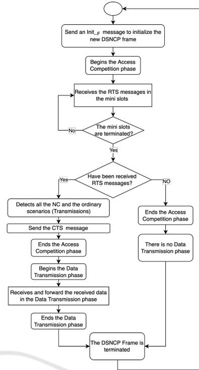
Figure 6: DSNCP flow graph for the relay node.
