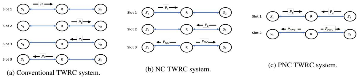
Figure 1: Three relaying schemes on a TWRC system: (a) conventional relaying, (b) NC scheme, (c) PNC scheme. Nodes  $S_1$  and  $S_2$  exchange packets  $P_1$  and  $P_2$  through the relay  $R$ .  $P_{NC}$  and  $P_{PNC}$ , respectively, represent the encoded packet resulting from NC and PNC technique.
