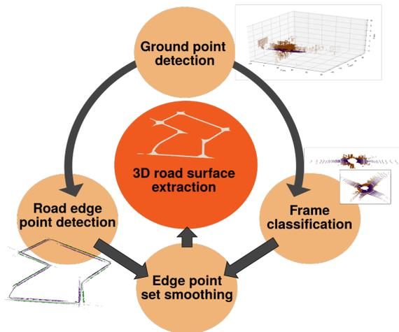
Figure 1: Summary of our proposed system, RoSELS, for 3D road surface extraction using ground points detected from an automotive LiDAR point cloud sequence. Our system includes two novel and significant intermediate processes of road edge point detection and frame classification.
