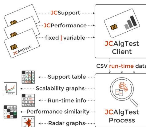
Figure 1: A high-level overview of the components and processes of our audit suite. The on-card applets measure the specification compliance and benchmark the performance. Then, the client collects and processes the results to extract a useful information.
