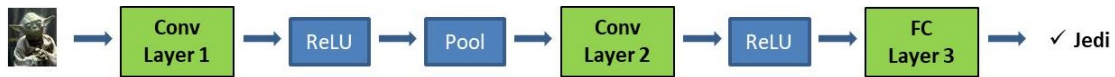
Figure 1: The example of a simple CNN. The green blocks are the linear layers (2 convolutional and one fully connected) and blue blocks are the non-linear layers.
