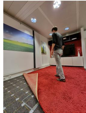
Figure 2: Test person walking on smart floor with visible wire pattern.
