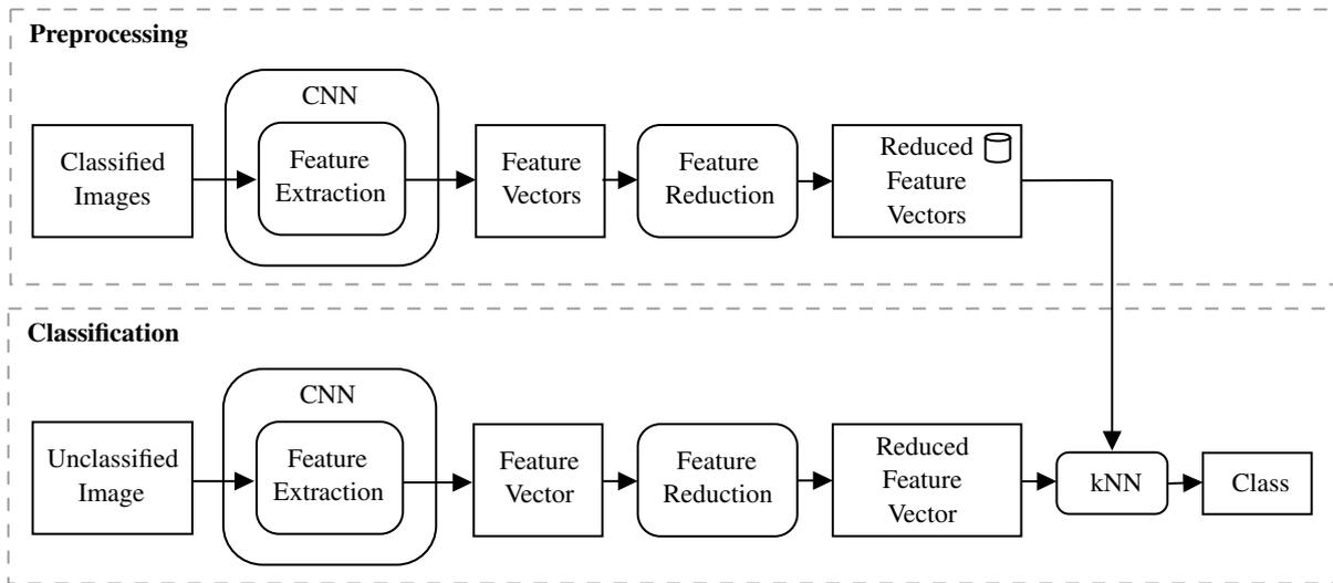
Figure 1: System for Product Image Classification based on Image Matching.
