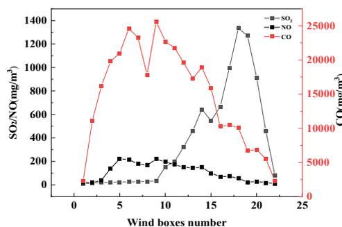
Figure 2: Distribution of smoke components in wind boxes.
