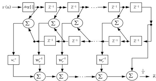
Figure 2: Realization structure diagram of 10kV High voltage digital electric energy metering verification device.
