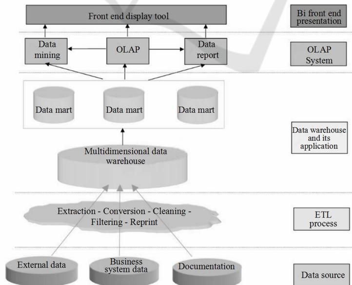
Figure 2: Functional structure diagram of business intelligence big data analysis platform.
