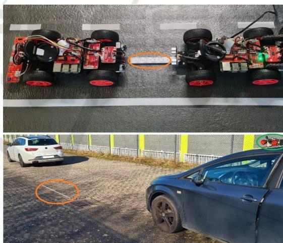
Figure 3: Manual data acquisition and annotation. Top: Distance measurements with model cars. Bottom: Distance measurements with real vehicles.
