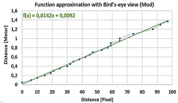
Figure 8: Function approximation with bird's eye view in a  $320 \times 160$  pixel image for model making data. Green line: Graph of an approximated linear function. Blue points: Real measured distances from data set 2 (Mod).
