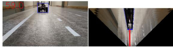
Figure 7: Bird's eye view transformation for data from model making area. Left: Input image with object detection and measured distance in pixels. Right: Transformed bird's eye view.
