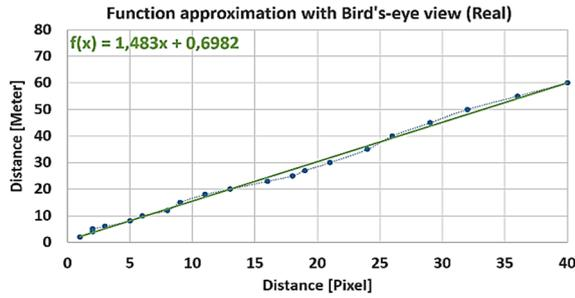
Figure 10: Function approximation with bird's eye view in a  $320 \times 160$  pixel image for real environment data. Green line: Graph of an approximated linear function. Blue points: Real measured distances from data set 3 (Real).
