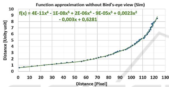
Figure 6: Function approximation without bird's eye view in a  $320 \times 160$  pixel image for simulation data. Green line: Graph of an approximated polynomial function of degree 6. Blue points: Real measured distances from data set 1 (Sim).
