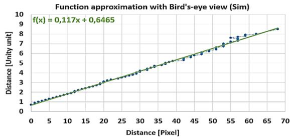
Figure 5: Function approximation with bird's eye view in a  $320 \times 160$  pixel image for simulation data. Green line: Graph of an approximated linear function. Blue points: Real measured distances from data set 1 (Sim).
