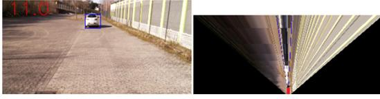
Figure 9: Bird's eye view transformation for data from real environment. Left: Input image with object detection and measured distance in pixels. Right: Transformed bird's eye view.
