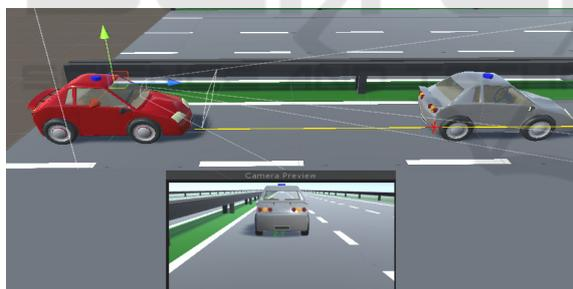
Figure 2: Automatic data acquisition and annotation with the Unity 3D simulator. Yellow line demonstrates the ray cast for the distance measurement (no. 1 in table 1).
