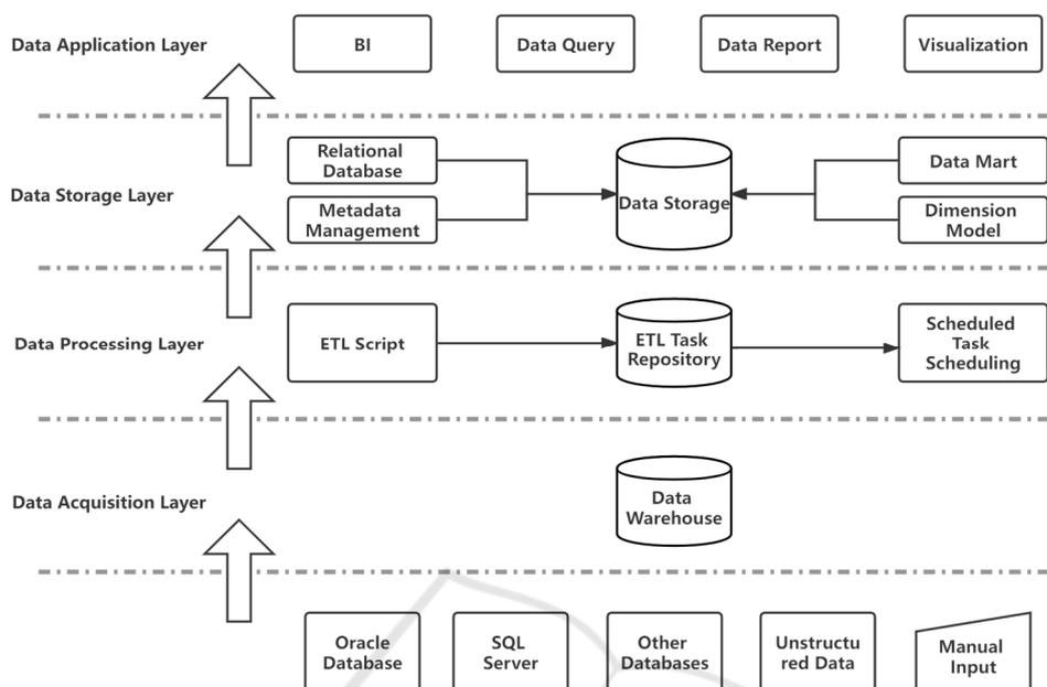
Figure 3: Design of a heterogeneous data warehouse architecture.
