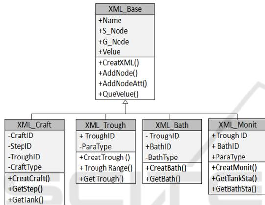
Figure 3: UML Diagram of XML layer functional class.
