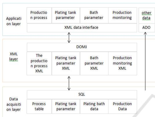
Figure 1: Digital electroplating production process information architecture.
